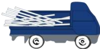
Incorrect way to load pipes
